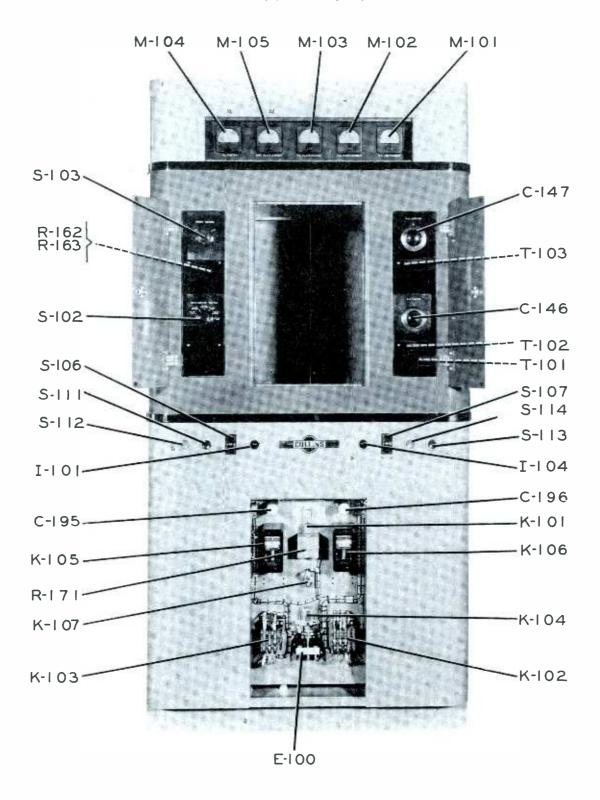
Figure 6-1. Transmitter Parts Arrangement, Front View
