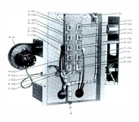
Figure 6-5. Audio Chassis Parts Arrangement
