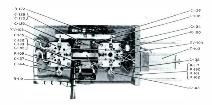
Figure 6-4. R-F Chassis Parts Arrangement, Bottom View
