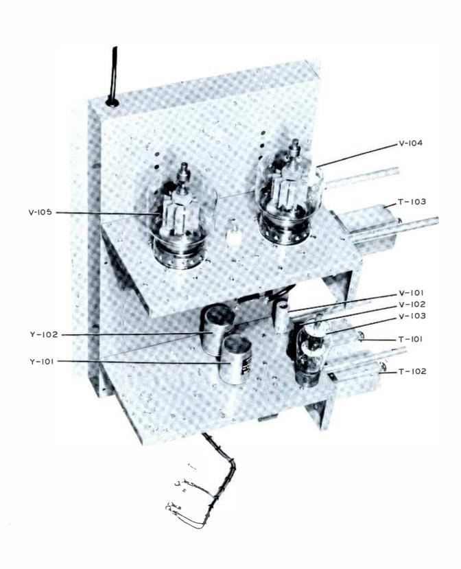
Figure 6-3. R-F Chassis Parts Arrangement, Top View
