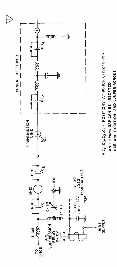
Figure 7-3. Arc-Supression Circuit Simplified Schematic
