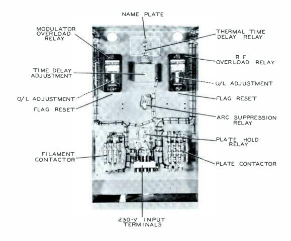
Figure 6-10. Relay Panel Controls
