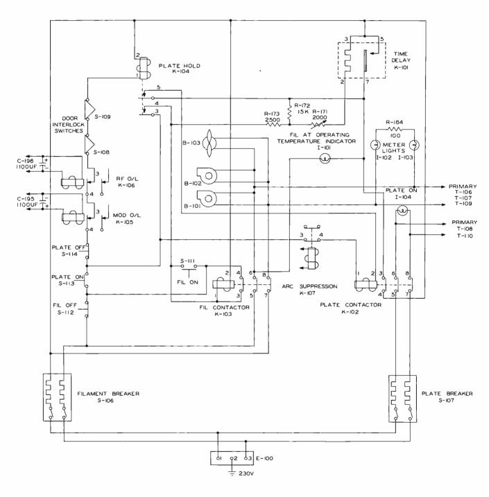
Figure 7-1. Primary Control Circuit Simplified Schematic
