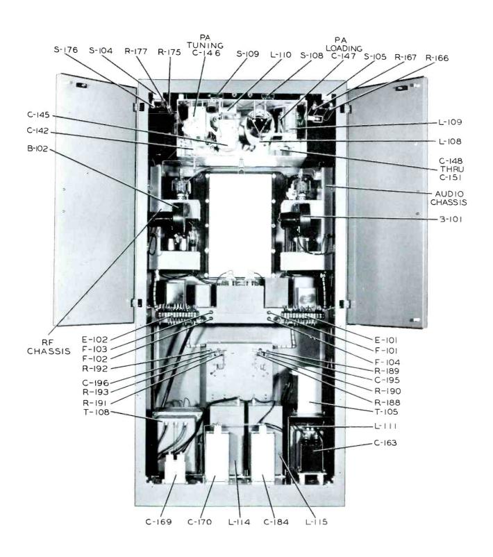
Figure 6-2. Transmitter Parts Arrangement, Rear View
