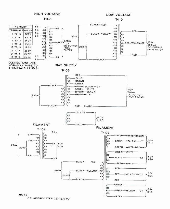
Figure 7-4. Transformer Details
