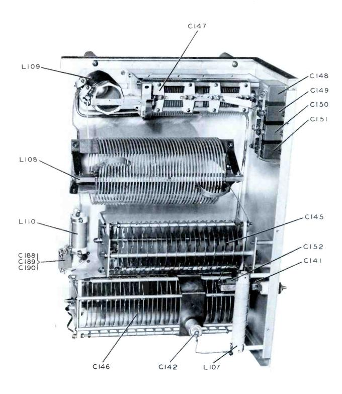
Figure 6-7. Output Network Parts Arrangement, Bottom View
