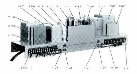
Figure 6-8. Power Supply Chassis Parts Arrangement
