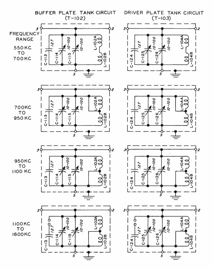
Figure 7-2. T-102 and T-103 Internal Connections
